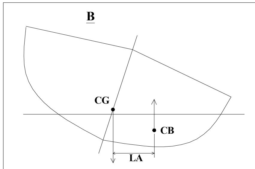
measured by the 'righting moment' which can be simply defined as the length of this lever arm, multiplied by the displacement of the boat, multiplied by the force of gravity. As the force of gravity is constant, it is fairly obvious that the longer the lever arm, the more stable a boat of a given displacement will be.
