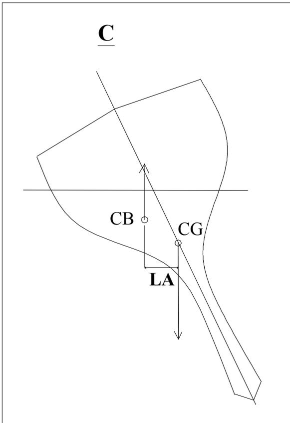
‘plank on edge’ hull style is not seen on today designs as it produced yachts which tended to be wet and sail at a heavy angle of heel. Modern ‘high tech’ racing yachts will combine high form stability with large quantities of ballast carried low down in bulb keels to obtain the best of both techniques.
